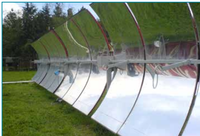
Figure 2. Parabolic concentrated solar power modules for industrial heat process Instituto de Investigaciones Eléctricas, Mexico
