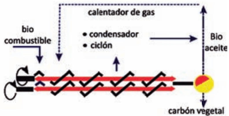
Figura 5.40 Reactor auger sin arena
